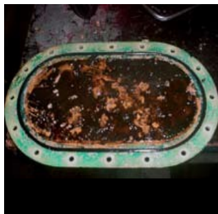
Figure 3. Microbial pollution of fuel tank
