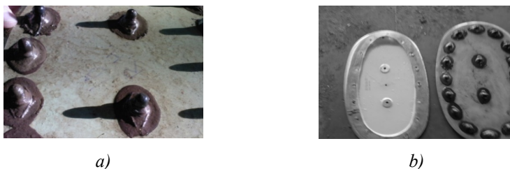
Figure 5 (a, b). Destruction of seals and hermetics by metabolites
