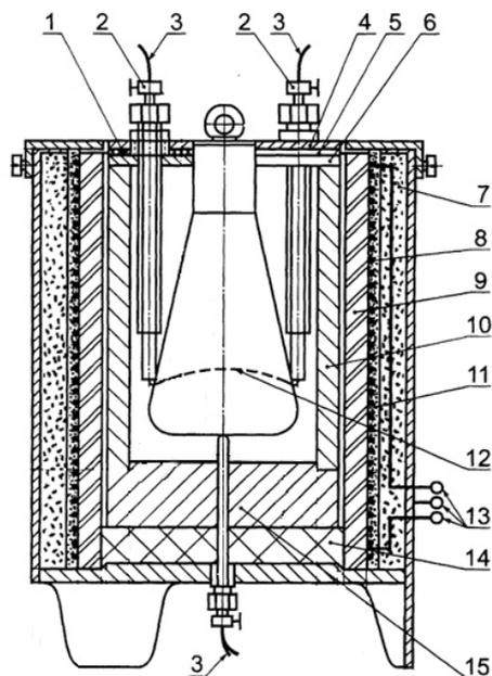
**Fig. 6.2.1. Test equipment for determining the ignition temperature of a gas:**
