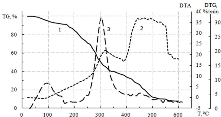
**Fig. 6.2.3. Curves of thermogravimetric (1), differential thermal (2) and differential thermogravimetric (3) analysis of sunflower husk**
