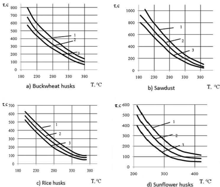
**Fig. 6.1.2. Dependence between heating temperature and moisture content for different types of processed biomass:**
