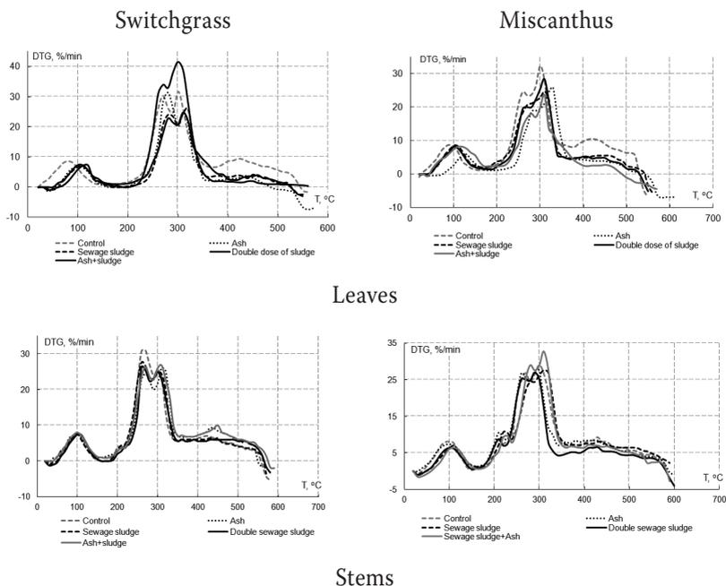
**Fig. 4.3.6. DTG curves of the thermal decomposition of Switchgrass and Miscanthus biomass**
