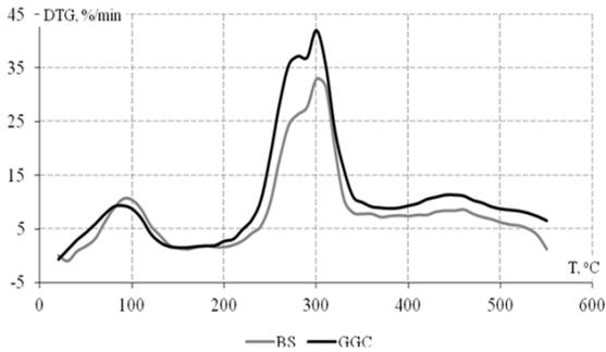
**Fig. 5.4.2. DTG curves of thermal decomposition of Populus wood**
