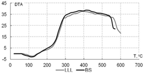
Fig. 5.4.5. DTA curves of Paulownia clone 112 wood thermolysis
