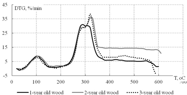
**Fig. 5.4.4. DTG curves of thermal decomposition of *Ailanthus altissima* wood**
