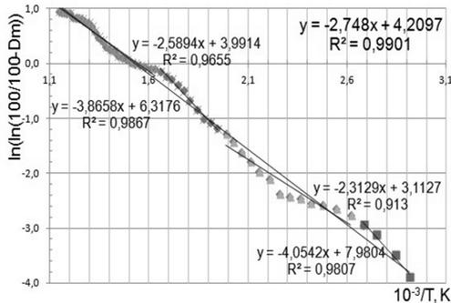
**Fig. 6.2.4. Diagram of the process of non-isothermal decomposition of sunflower husk**
