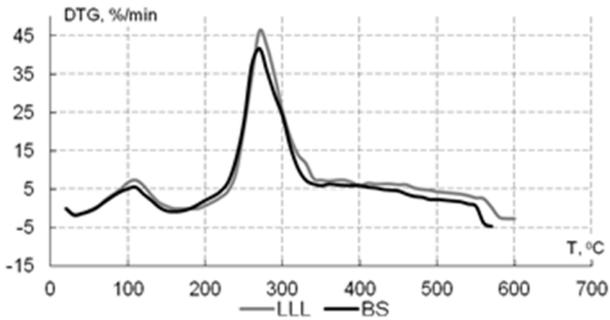
Fig. 5.4.6. DTG curves of Paulownia clone 112 wood thermolysis
