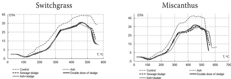
**Fig. 4.3.7. DTA curves of the thermal decomposition of Switchgrass and Miscanthus leaf biomass**
