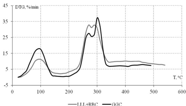
Fig. 5.4.1. DTG curves of thermal decomposition of Elaeagnus wood
