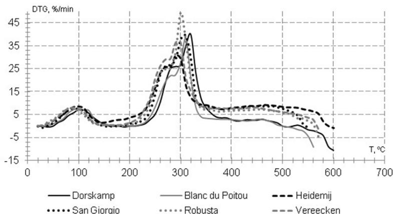
**Fig. 5.3.2. DTG curves of poplar wood thermal decomposition**
