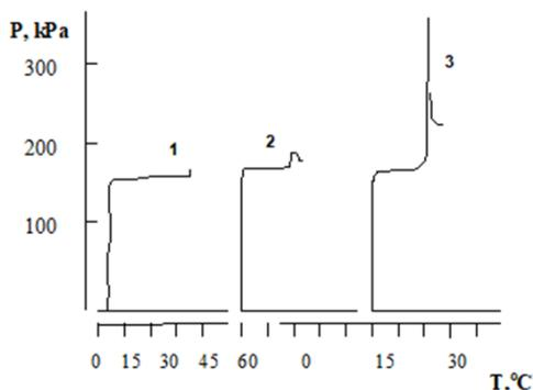
**Fig. 6.2.7. Barograms of studies at a temperature of 490 °C with O<sub>2</sub> = 42.3 %: 1 – no ignition; 2 – degenerate ignition; 3 – self-ignition**
