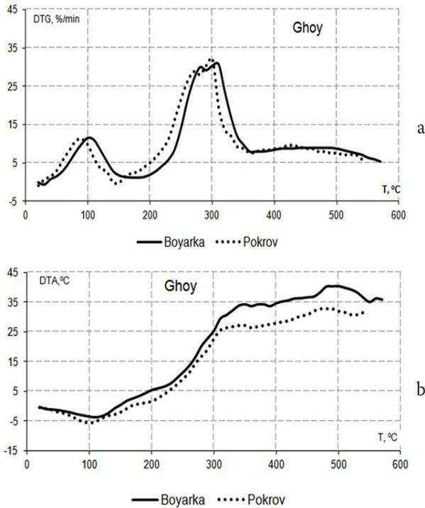
**Fig. 5.3.4. DTG and DTA curves of “Ghoy” poplar clone wood thermal destruction in Boyarka and Pokrov stations**
