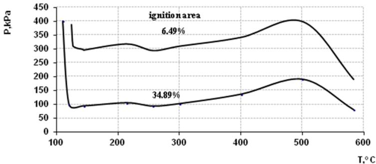
**Fig. 6.2.9. Dependence of the autoignition temperature on pressure for a gas mixture with air**
