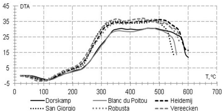
Fig. 5.3.1. DTA curves of poplar wood thermal decomposition
