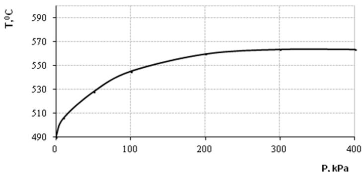
**Fig. 6.2.8. Dependence of the autoignition temperature on pressure**
