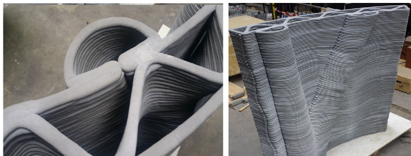
Figure 4. 3D-printed wall structure
