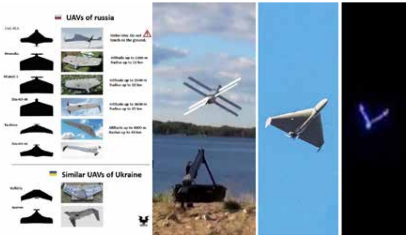
Figure A.2.40 – Main aircraft-type UAVs used by Russia and Ukraine. Lancet UAV; UAV Shahed-136 (Heran-2)
