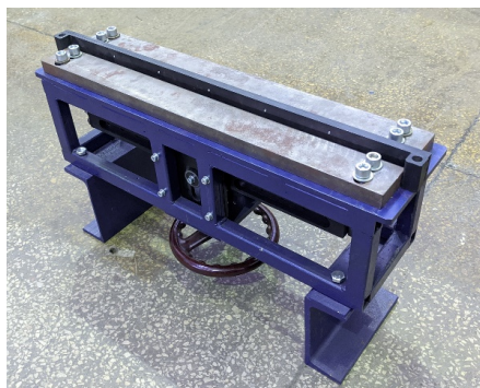
Fig. 18. Clamping device for welding flat and cylindrical samples made of thin sheet material
