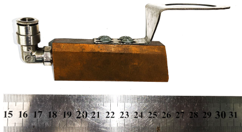
Fig. 15. Manufactured gas protection device for welded joints
