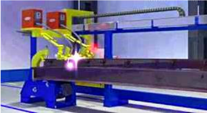
Figure 1. Basic technology for producing a spine beam without deflection at the prestressing stage
